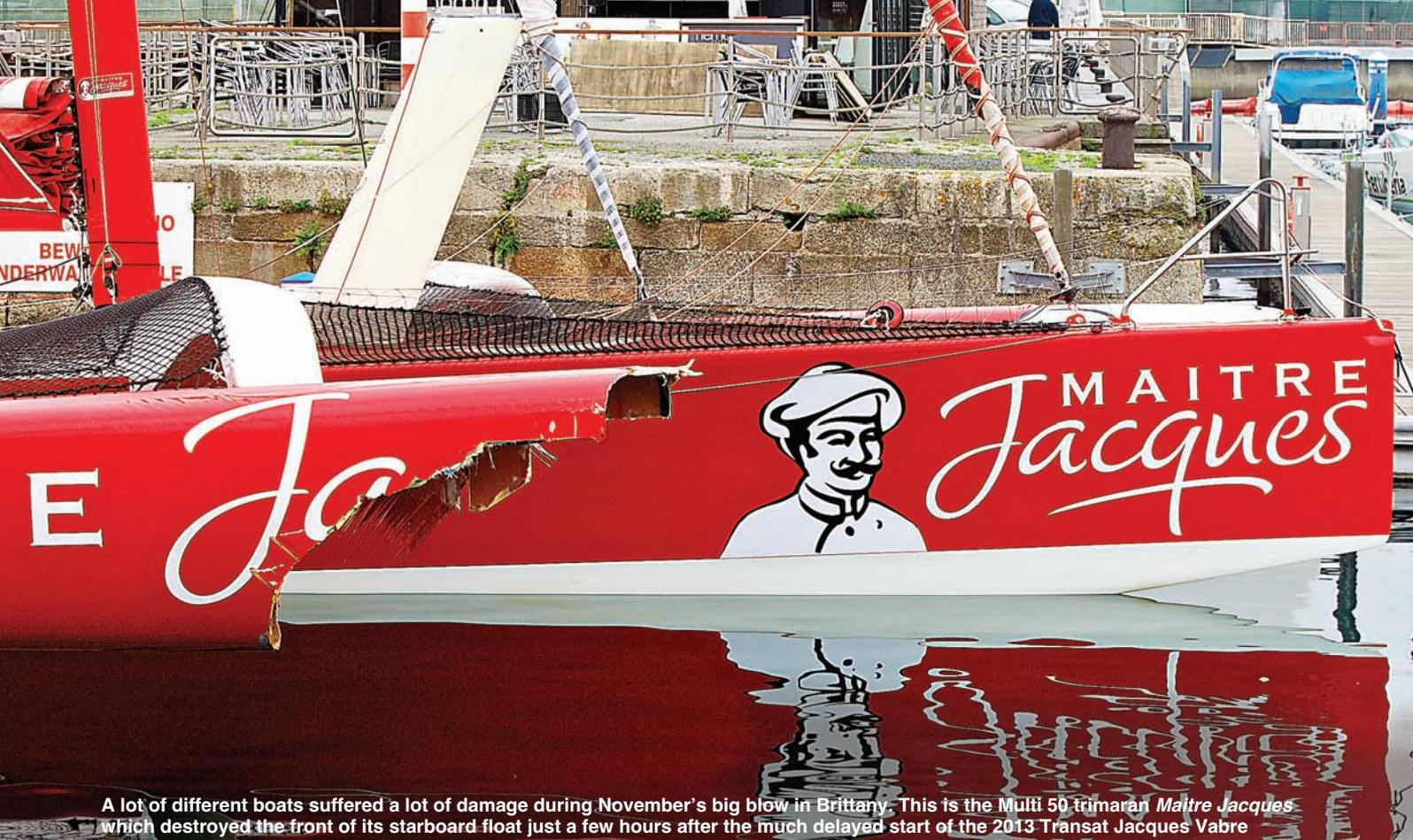
A lot of different boats suffered a lot of damage during November's big blow in Brittany. This is the Multi 50 trimaran *Maitre Jacques* which destroyed the front of its starboard float just a few hours after the much delayed start of the 2013 Transat Jacques Vabre
