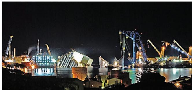
**Salvage engineering on a giant scale. Empty, the displacement of the *Costa Concordia* exceeded 114,000 tons before factoring in the vast weight of water trapped in the wreck. The original tear in the hull bottom was more than 50m making a patch-up impossible. Now that she is upright once again work is underway to refloat the vessel – with the final removal to a scrapyard scheduled for spring 2014**
